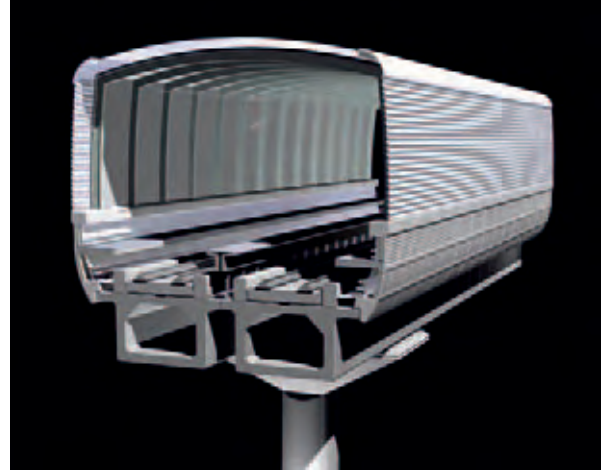
12. Design for full noise enclosure at crossings.
